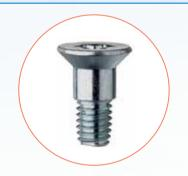
The finished product delivered by Bossard is a specially made screw that has a thread diameter of 4.5 mm. It cuts the thread the first time it is inserted and it comes with a special supporting shank. The Torx® drive prevents damage to the screw head at high torques. The underlying round flange holds the chair parts together securely.
