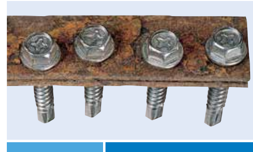
ecosyn®-MRX self-cutting screws after 1,500 hours testing in the salt spray: from head to tip, no trace of any corrosion anywhere
